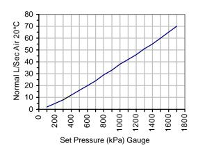
Discharge Capacity measured at 10% over set pressure
